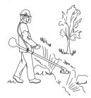
5 Take great care when cutting a tree that is in tension. A tree that is in tension may spring back to its normal position before or after being cut. If you position yourself incorrectly or make the cut in the wrong place the tree may hit you or the machine and cause you to lose control. Both situations can cause serious personal injury.
